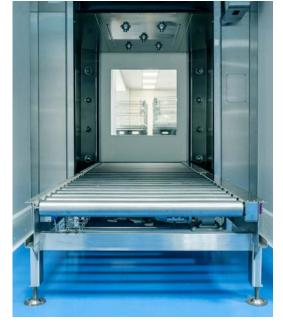
Material handling systems are manufactured in stainless steel AISI 304 or 316, both structure (frames, covers) and mechanics (rollers, chains, sprockets).
