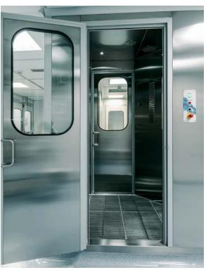
Misty decontamination water shower operates through the action of water spray which dampens the operator clothing (generally made in Tyvek), to adhere powders, without getting him wet.
